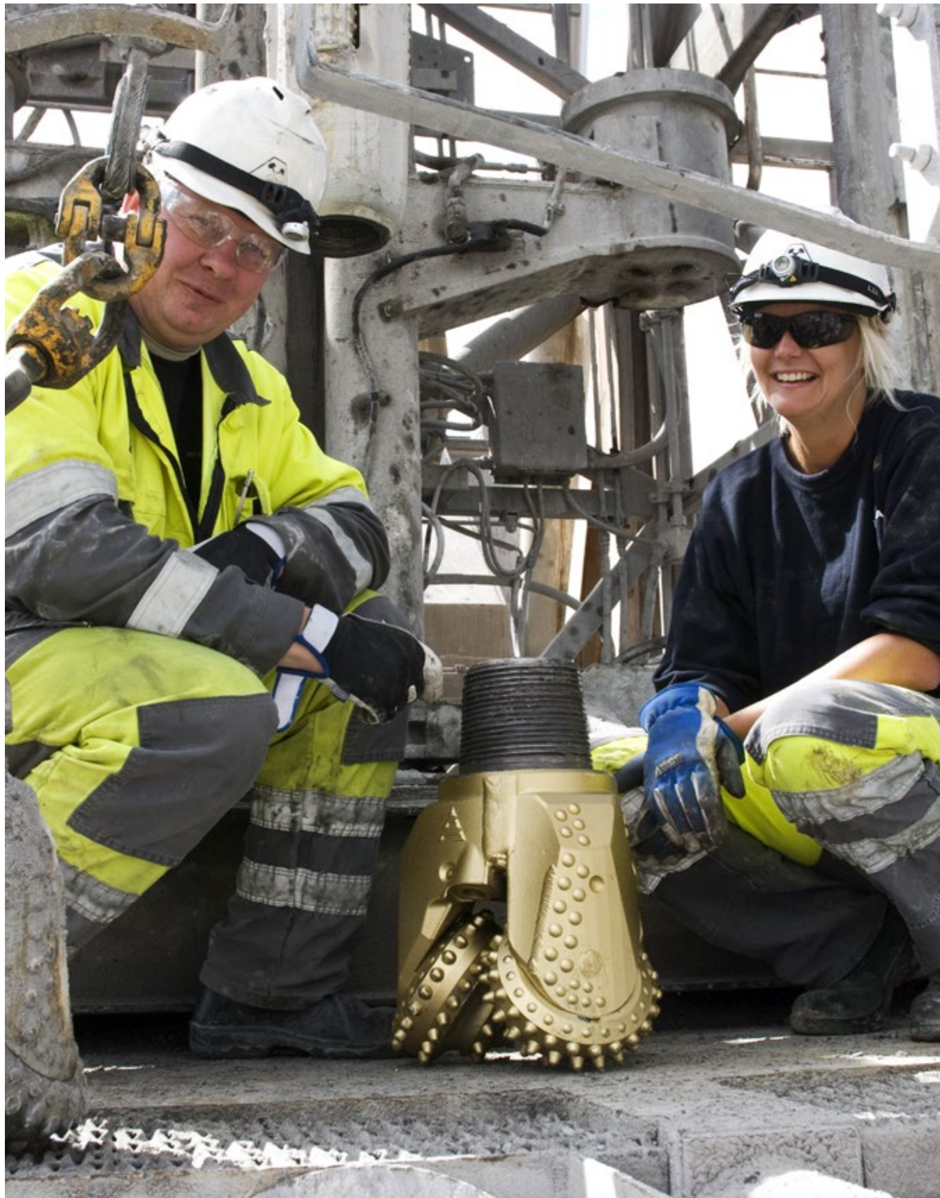
Changing a drill bit at Titania's open cast mine at Tellenes in Rogaland. Photo: Titania AS /Linda Løvås
