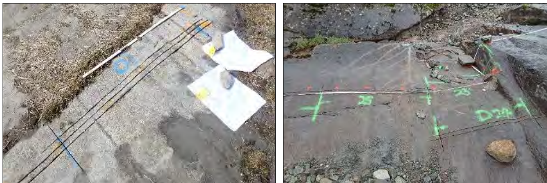
Figure 3-15 Examples of field duplicate samples using the opposing side of the channel (left) or a parallel sample (right)
