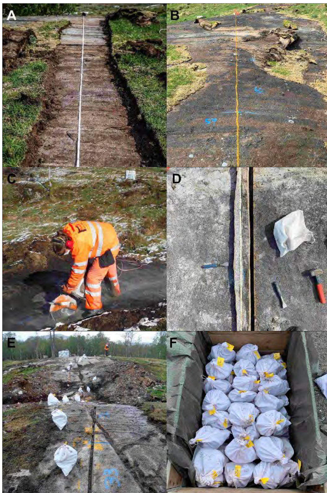
Figure 3-3 Channel sampling method
